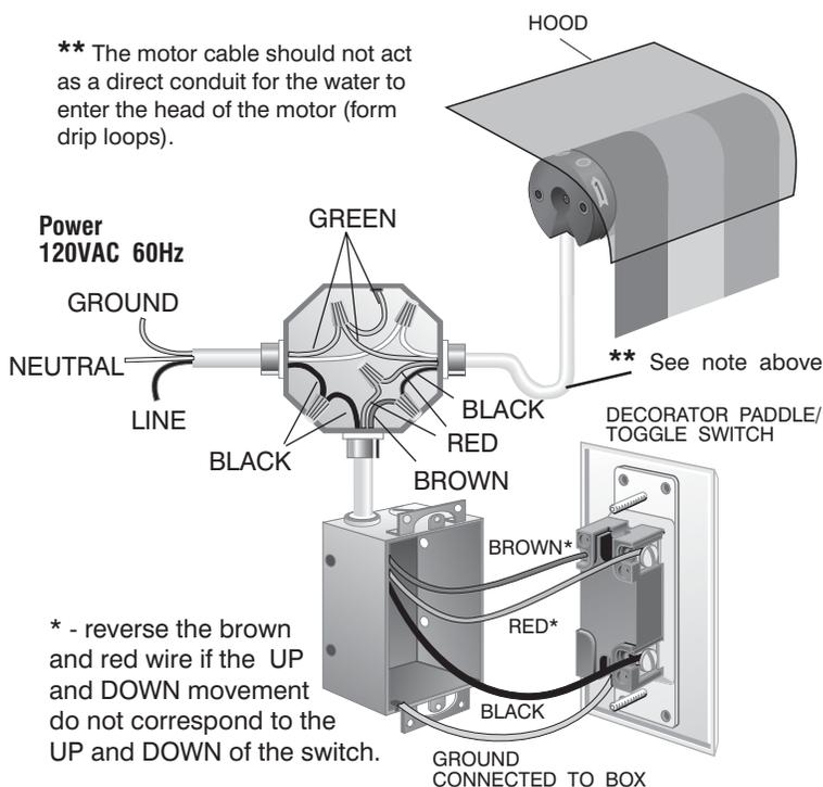
\* - reverse the brown and red wire if the UP and DOWN movement do not correspond to the UP and DOWN of the switch.
