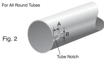
**Notch: LS40** Length =  $\frac{A}{.335 / 8.5}$  in./mm      Width =  $\frac{B}{.236 / 6}$  in./mm
